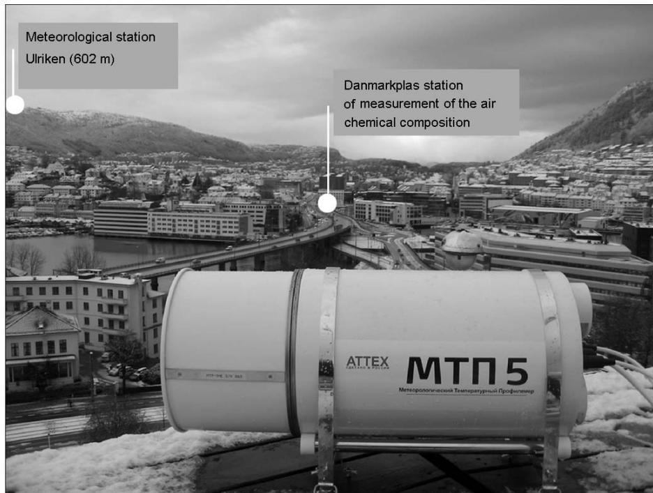
**Fig. 1.** Meteorological temperature profiler produced by NPO ATTEX (Russia, [www.attex.net](http://www.attex.net)). The instrument is installed on the measurement site of the Geophysical Institute of University of Bergen at the height of 45 m above the sea level. The image is dated from February 8, 2011.
