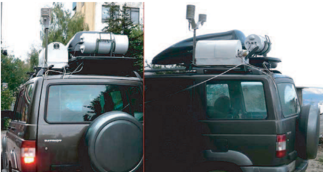
Figure 1: Mobile microwave system installed on UAZ “Patriot”.
